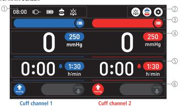
The main screen is divided up into 1 status bar, 2 control bar, 3 channel bar, 4 pressure display, 5 time display and 6 inflation / deflation area.
